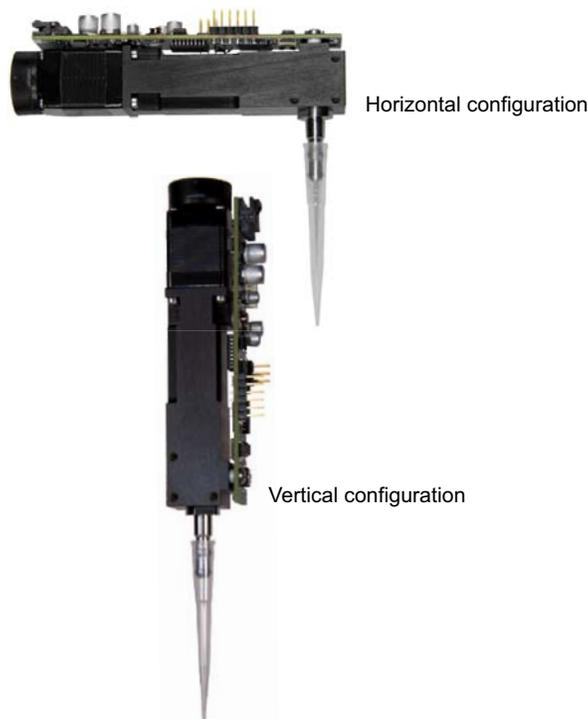
The Air-Z Flex Air Displacement Pipette Pump is a full-featured, fully programmable air displacement pipette module designed for automated instrumentation. Utilizing disposable tips, cross contamination and carryover during sample transfer and reagent aliquoting are avoided; and the tubing and priming normally required for liquid handling are eliminated.
