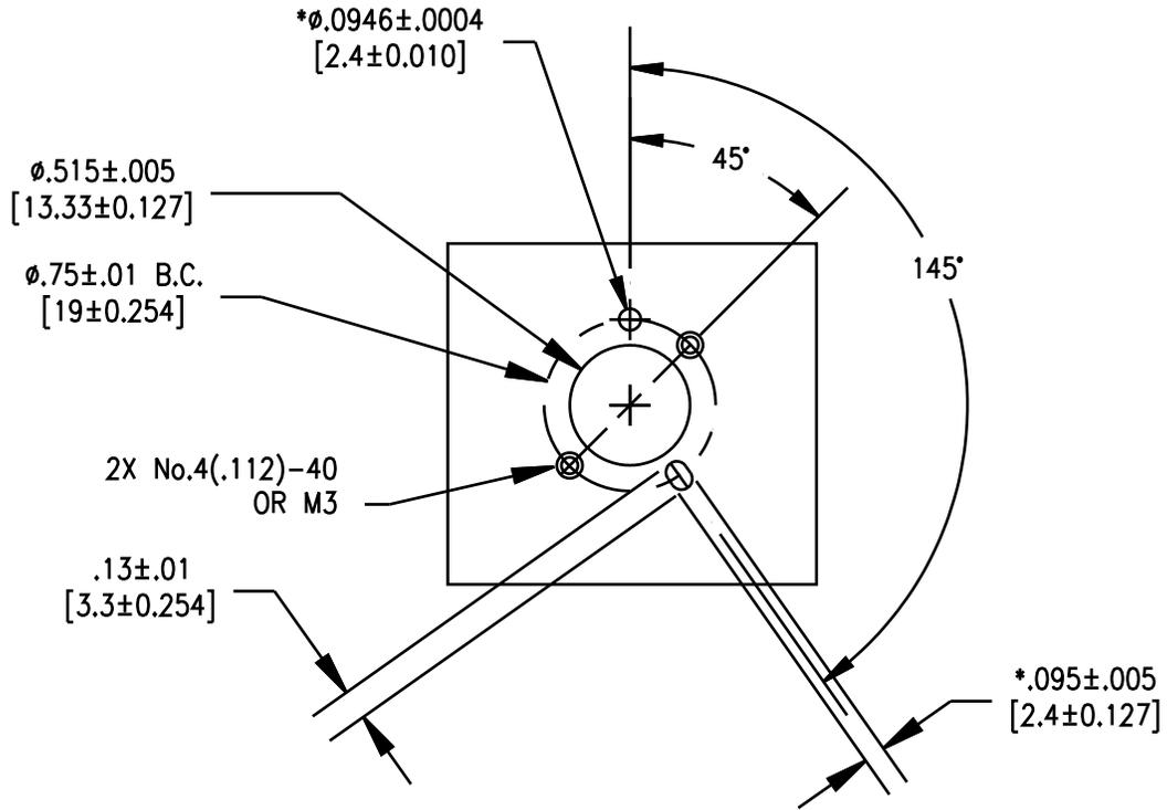
\*NOTE: THESE DIMENSIONS ARE ONLY NEEDED WHEN THE VALVE IS INTERFACED WITH A SYRINGE. FOR VALVE ONLY MOUNTING, USE  $\phi.098$  [2.5mm] OR LARGER HOLES.
