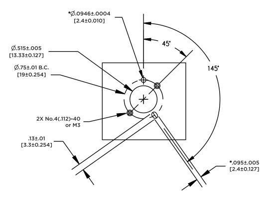
\*NOTE: THESE DIMENSIONS ARE NEEDED WHEN THE VALVE IS INTERFACED WITH A SYRINGE. FOR VALVE ONLY MOUNTING, USE  $\emptyset$ .098 [2.5] OR LARGER HOLES.
